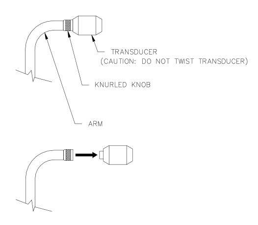
FIGURE B-1. CA27 Transducer and Arm
